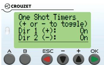
This screen allows for the two one-shot timer settings to be enabled or disabled. This setting prevents access control from holding a direction open on the standard direction inputs. Toggle Directoin1 by pressing + and Direction 2 by pressing -. This should be set to "On" in almost every installation.
