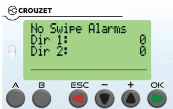
This screen lists how many times the alarm went off because the arm was approached without swiping (whether while closing or while in the closed position).
