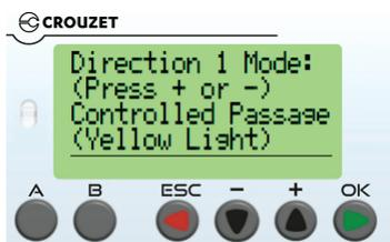
The value on this screen defines the standard operation of direction 1. It can be set to Controlled Passage (w/ yellow indicator lights), Free Passage (w/ green indicator lights) or No Passage (w/ red indicator lights). Controlled or Free are the most common settings, but if there are multiple lanes, using No Passage may help to spread traffic through multiple lanes. This is configured based on our understanding of the job requirements in the factory, but can be cycled by pressing the + button.
