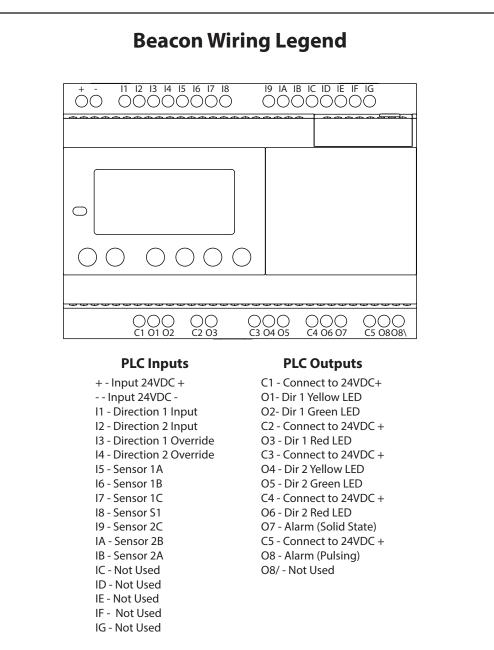
All inputs are PNP type transistor inputs - apply local 24VDC + to terminal for PLC to register.
