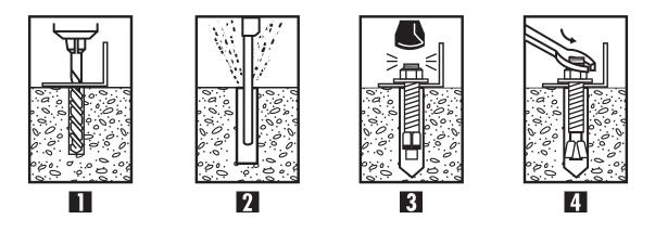
Select a carbide drill bit with a diameter equal to the anchor diameter. Drill hole at least 1/4" deeper than nominal anchor embedment.
