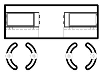
Loosening the screws holding the bracket to the panel will allow for some range of motion up and down.
