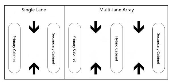
From the factory, each cabinet in an array is preconfigured to the requested operation and layout. Each lane has two directions of passage, each of which can be configured for controlled passage, free passage or no passage. This configuration can be changed in the field via settings on lane's logic controller located inside of the primary cabinet.
